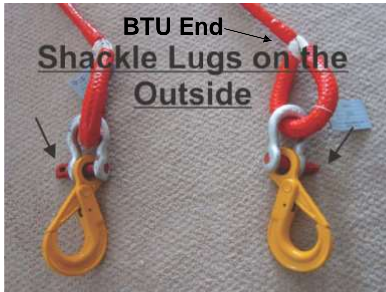
Figure 10: Self-Locking Hooks Installed on BTUs
