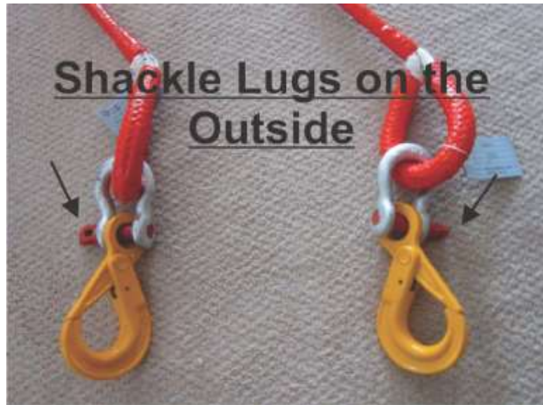
Figure 26: Self-Locking Hooks Installed on BTUs
