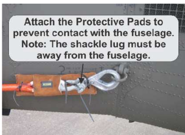
Figure 18: Attach Anti-Chafe Pad
