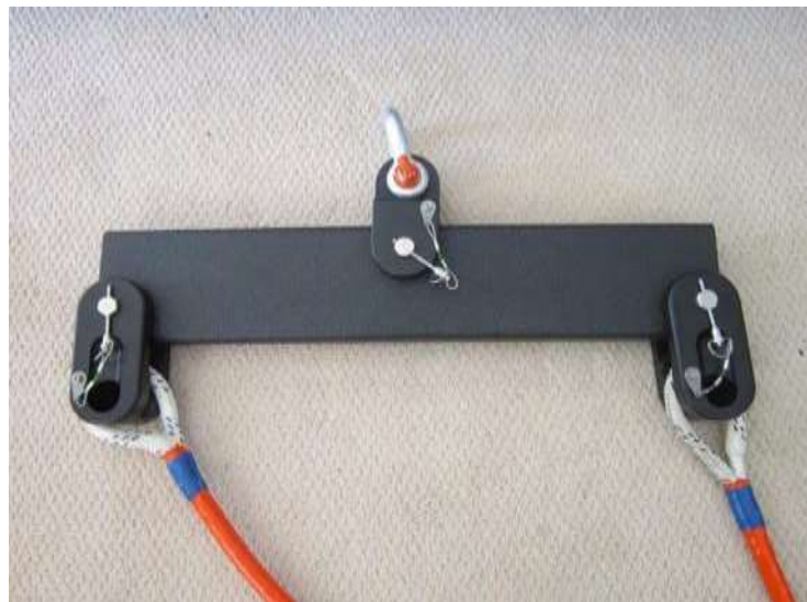
Figure 16: Proper Assembly of Adapters w/ Ropes
