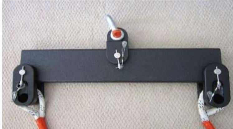
Figure 9: Proper Assembly of Adapters w/ Ropes
