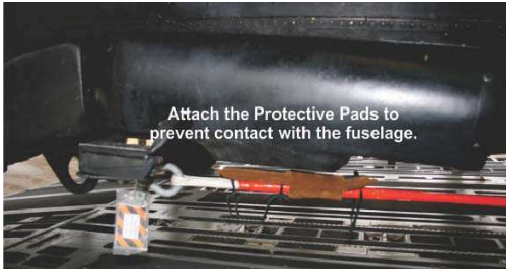
Figure 13: Anti-Chafe Pads Installed
